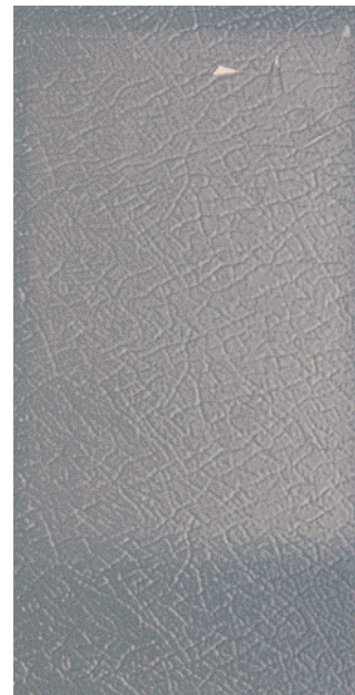
Proprietary plastisol on HDG
