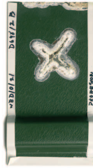
Proprietary plastisol on HDG
